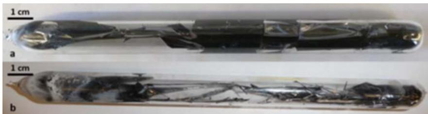
Figure 1. Various photographs of the unopened quartz reaction tubes with black metallic flakes of directly-synthesized PC<sub>x</sub> deposited on the walls and as free-standing flakes.
